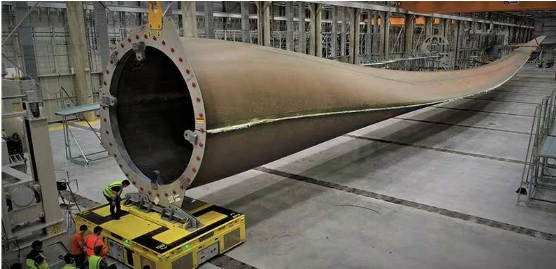
Wind turbine blade 107 meters in length (Cherbourg, France)
